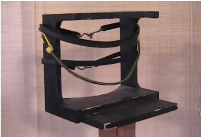
Board holder was made from \frac{3}{4} inch plywood. It was cut to fit the curvature of the 75 lb. bag and was attached with rubber bungee cords.
