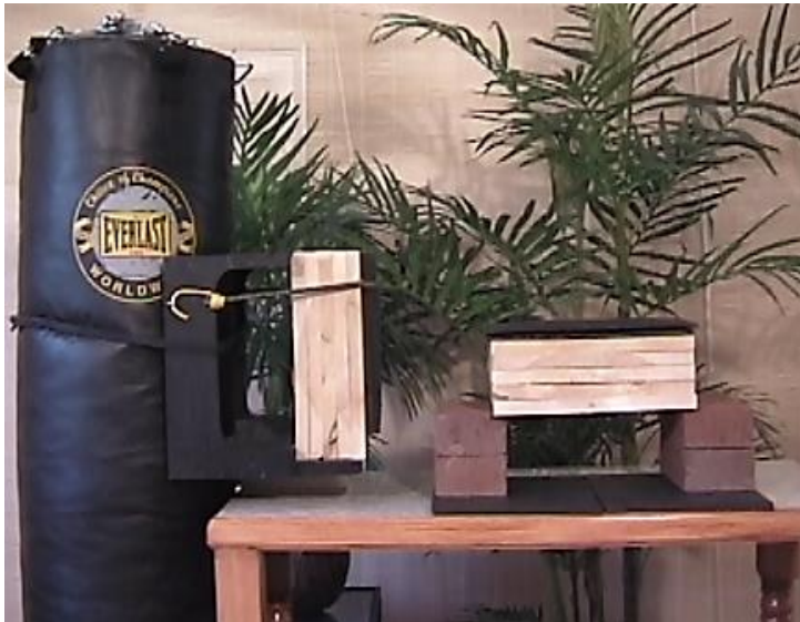
The 5 suspended boards (left) are considerably more difficult to break than the 5 rigidly supported boards on the right.
