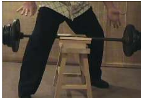
Test boards must support a 130 lb. barbell for 1 full second, then break with 135 lbs.
